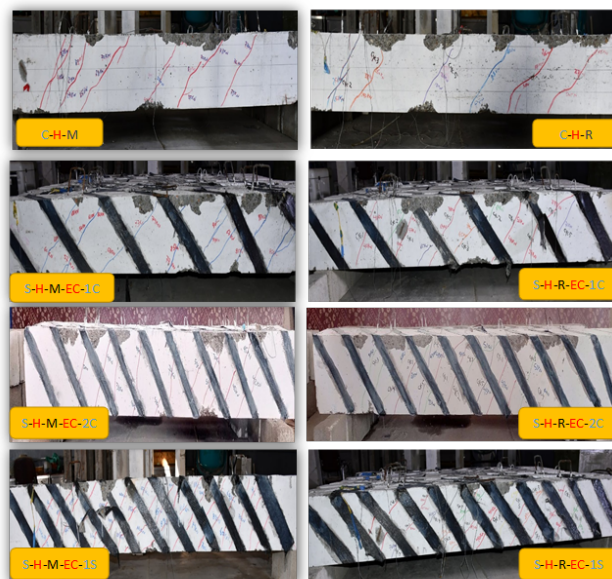
Fig. 23. Failure modes of beams tested under monotonic and repeated loads.
