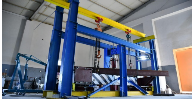
Fig. 5. Testing setup with the loading frame.
