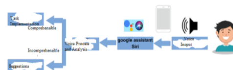
Fig.1: The implementation mechanism of voice command
