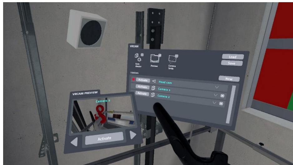
Figure 2. Virtual camera tools inside a virtual elevator shaft. Using the VRCAM menu, the presenter can create a set of virtual cameras (white box) and save or load the set. They can preview and activate the view from each camera using a preview window attached to their VR controller (VRCAM PREVIEW). The first-person view was captured from a stabilized virtual camera attached to the presenter's head (headcam).
