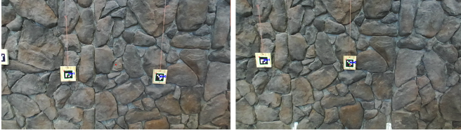
Fig. 7. The left image shows the initial pose of the camera, whereas the right image shows a control result of driving the TCP (image center) to a specific marker.
