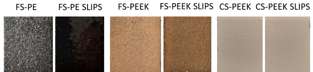
Figure 1. FS-PE, FS-PEEK and CS-PEEK coating surfaces before and after oil impregnation (SLIPS). Sample size is 30 × 40 mm.
