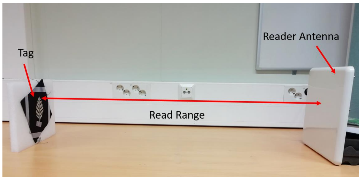
Figure 3. Practical testing setup in an office environment, a tag with a leaf-shaped antenna attached to a foam fixture.
