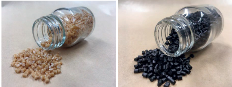
Figure 14: The wood-plastic composite pellets containing 20 wt% of wood flour (PP-W20) and wood-plastic composite pellets containing 20 wt% wood flour and 15 wt% graphene nanoplatelets (PP-W20-G15)
