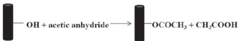
Figure 6: Schematic representation of acetic anhydride modification of lignocellulosic fibre [59, 60]
