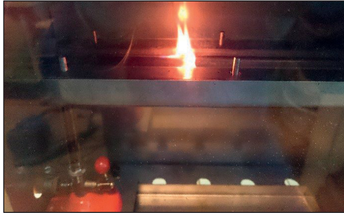
Figure 15: A viscose fabric/epoxy composite sample tested for determining the burning rate
