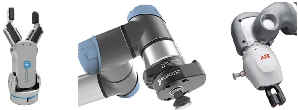
Figure 6. On robot two finger gripper [76], Robotiq vacuum gripper [77] and ABB smart gripper [78] with vacuum and two fingers combined
