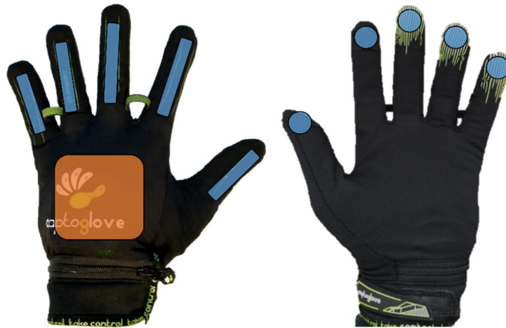
Figure 7. Locations of the sensors, on left palm side down picture the bending sensors and pressure sensors in right palm side up picture are presented in blue color and the transmitter is presented in orange color
