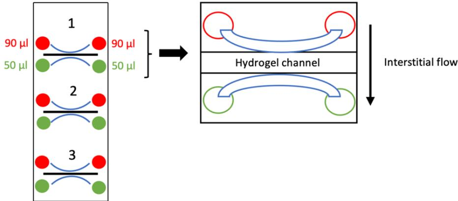
**Figure 3.** A schematic picture of the AIM Biotech 3D Cell Culture Chip structure showing how the interstitial flow is created. By adding different volumes of medium to the upper (red) and lower (green) medium reservoirs, hydrostatic pressure is created and the medium flows through the hydrogel channel creating interstitial flow. (AIM Biotech, viewed 16 April 2021, <https://aimbiotech.com/product/3d-cell-culture-chips-3dt/>)
