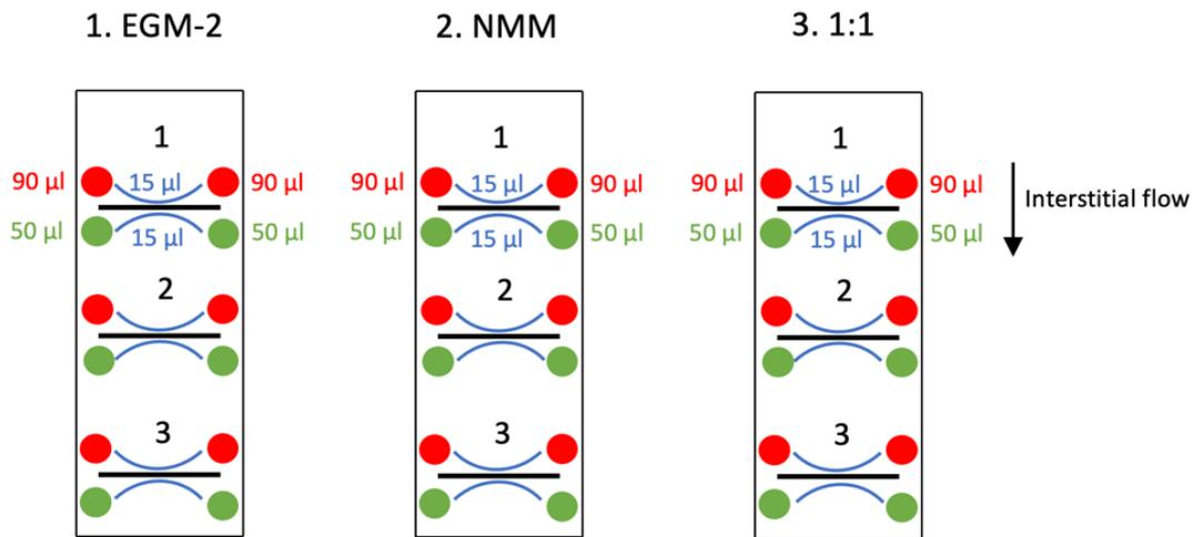
**Figure 5.** A schematic image of the media volumes added to the AIM Biotech chips. First, 15  $\mu\text{l}$  medium is added to the medium channels (blue). Second, 90  $\mu\text{l}$  medium is added to the upper medium reservoirs (red) and 50  $\mu\text{l}$  medium is added to the lower medium reservoir (green) to create the interstitial flow. Used medium: Chip 1. = EGM-2, Chip 2. = NMM, Chip 3. = 1:1 mixture of EGM-2 and NMM.
