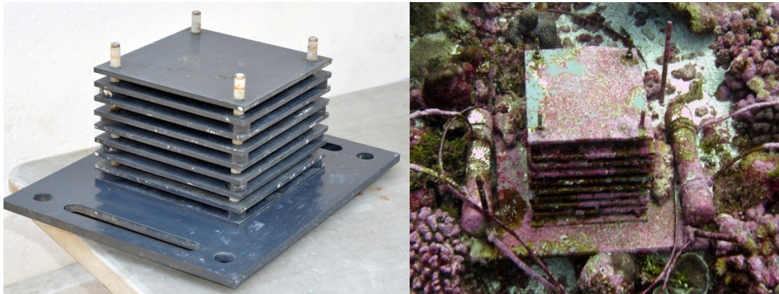
Figure 2. Autonomous Reef Monitoring Structure Unit before and 2 years after deployment
