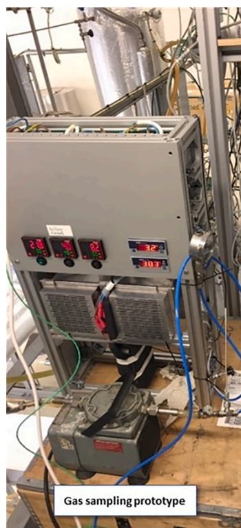
Fig. 4. ACEMS prototype for online liquid and gas monitoring in operation at the SINTEF pilot plant (left picture). Right picture showing the mass spectrometer setup connected for analysing condensate from to the gas sampler.
