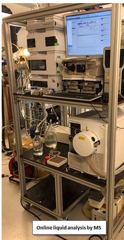
Fig. 4. ACEMS prototype for online liquid and gas monitoring in operation at the SINTEF pilot plant (left picture). Right picture showing the mass spectrometer setup connected for analysing condensate from to the gas sampler.
