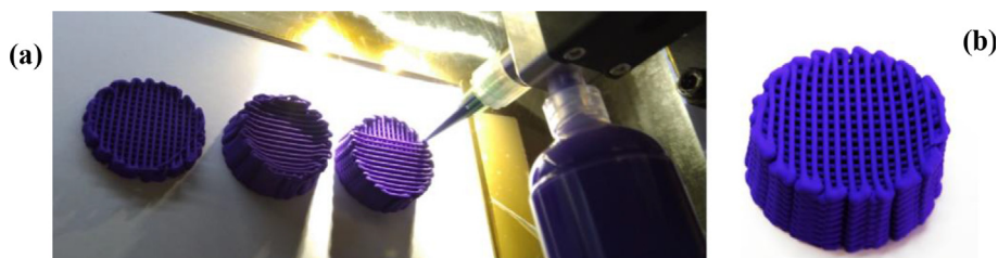
Fig. 1. 3D printed UTSA-16 monoliths: (a) consistent periodic structures produced by tuning the formulation and nScript 3D printing parameters and (b) image of an as-fabricated cylinder with a diameter of ca. 2.5 cm after drying.
