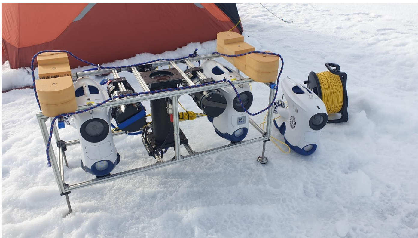
Figure 54. On the left, the double Blueeye and on the right the Blueeye are ready to be deployed in the water. The tent on the back served as control room for the vehicles.
