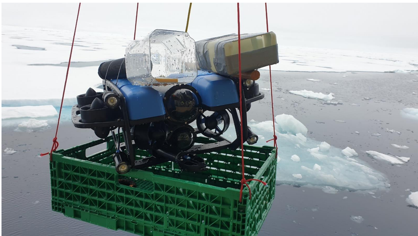
Figure 58. Blue Robotics ROV tested with sampling devices 2 and 3 at the same time. In this case the difference in hydrodynamics and buoyancy between the designs made the vehicle difficult to manoeuvre and to have a constant roll.
