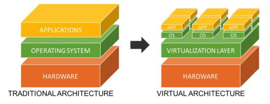
Figure 2.2 Traditional Computing Architecture vs Virtual Architecture
