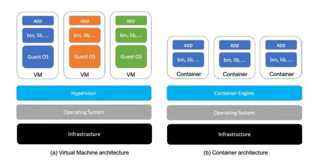
Figure 2.4 VM architecture vs Container architecture
