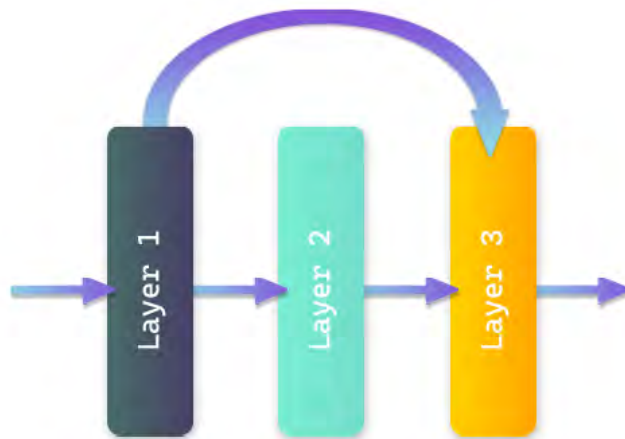
Figure 2.7: A simple example of residual neural network where layer 2 is skipped by layer 1.
