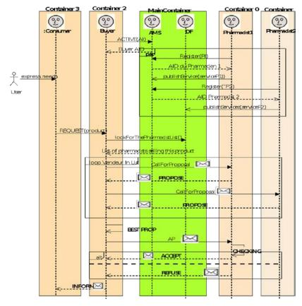
Fig. 20: Detailed protocol diagram of the "Drug Purchase Negotiation" capability
