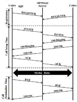
This protocol is dependent on internet protocols but independent of transport layer. A SIP based session or application consists of three stages. i. The Registration ii. The Initiation and iii. The Termination. The working of these stages depends on SIP proxy server for connectivity between nodes. The application performance is mostly affected due to delays which occur in the process of these stages. The acceptable average delay in a SIP system is in the range of [0.145, 0.345] seconds.
