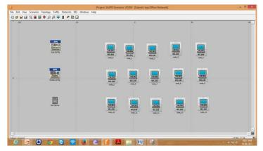
Our main concentration is towards VoIP QoS, so mobility in nodes is ignored and are restricted to static model. The entire network is configured to function as VoIP network with GSM application and voice codec as G711. Different scenarios have been created for different MANET routing protocol but the topology, application configuration and other parameters have been kept constant so that we obtain an ideal comparision among the protocols used.
