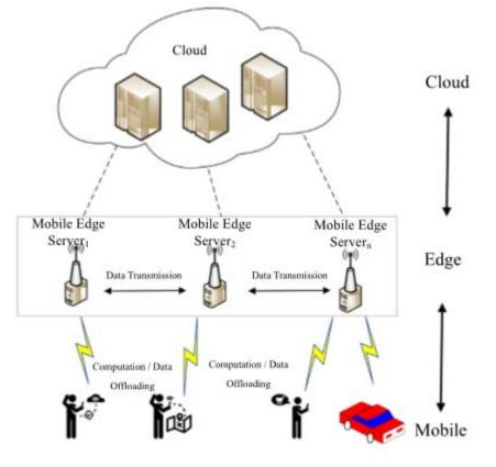
*Figure 1:* A typical mobile edge computing architecture [6].
