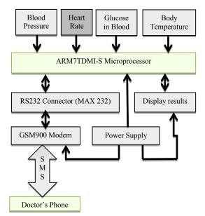
Figure 7 : Implementation of the complete system of patient monitoring system
