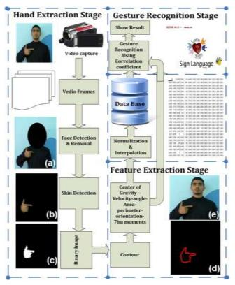
*Figure 1 :* Gesture recognition system architecture (a) Face detection and removal, (b) Hand extraction using YCbCr skin color detection Algorithm, (c) Hand extraction with binary image, (d) The contour of the hand blob & (e) The center of gravity
