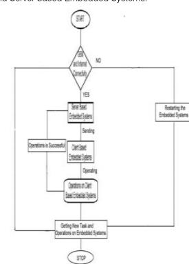
Flow Chart Diagram of Embedded System
