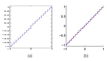
*Fig. 2:* Proposed Quantizer with K=0.8 and M=0.3 (a) Quantization curve (b) De-quantized values
