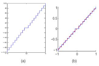
*Fig. 1:* Existing Quantizer (a) Quantization curve (b) Dequantized values
