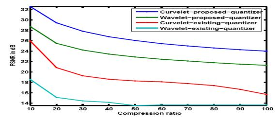
*Fig. 4:* PSNR Vs Compression ratio corresponding to Wavelet with existing quantizer, Curvelet with existing quantizer, Wavelet with proposed quantizer and Curvelet with proposed quantizer for Barbara image
