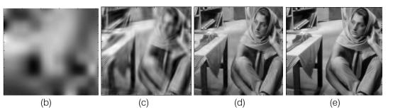
*Fig. 3:* Barbara image for compression ratio of 1:20 (a) Original image (b) Wavelet with existing quantizer (c) Curvelet with existing quantizer (d) Wavelet with proposed quantizer (e) Curvelet with proposed quantizer
