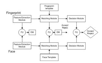
Figure 2 : Multimodal Biometric System using Face & Fingerprint
