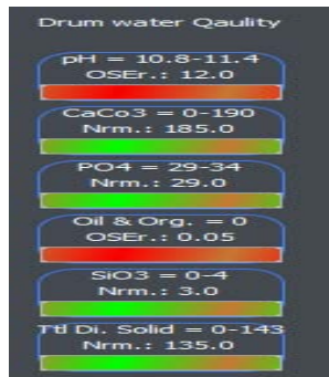
Figure 9: Drum Water Quality Display Panel
