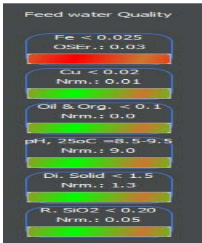
Figure 13: Feed Water Quality Display Panel
