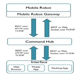
*Figure 2:* The System Communication Protocol
