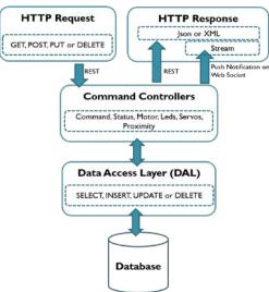
Figure 3: Command Hub Architecture
