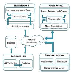
Figure 1: The System Architecture
