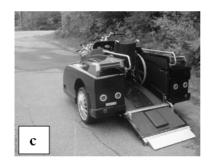
Figure 1: Products available for wheelchair users as drivers remaining seated in their wheelchairs: a) one place car (source: http://www.kenguru.com), b) up to three places for wheelchair users (source: http://www.soul-emotion.fr) and c) motorcycle (source: http://www.mobilityconquest.com).
