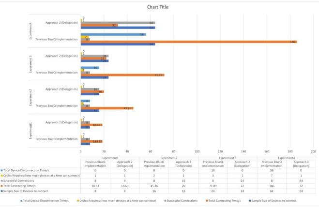
Figure 11: Approach2 VS. BlueQ - Test Results
