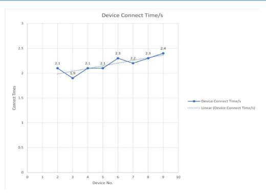
*Figure 9:* Approach2 (Delegation) – Test Results(Client Device)
