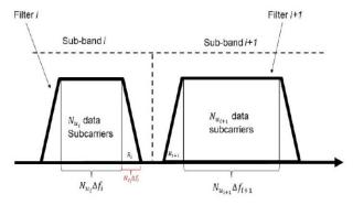
Figure 5: Role of transition bands of the filter
