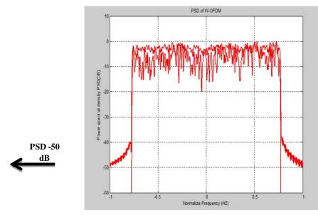
Figure 8: Power spectral density (PSD) of W-OFDM
