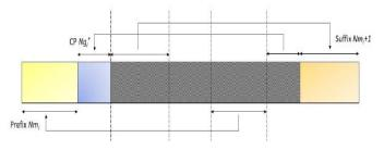
*Figure 2:* CP, prefix and suffix extension for a W-OFDM symbol
