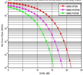
Figure 15: BER for MIMO-OFDM, MIMO-WOFDM and MIMO-FOFDM over Rayleigh fading channel using 16-QAM
