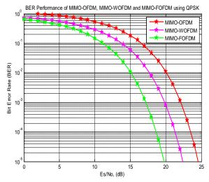
Figure 11: BER For MIMO-OFDM, MIMO-WOFDM and MIMO-FOFDM over Rayleigh Fading Channel using QPSK
