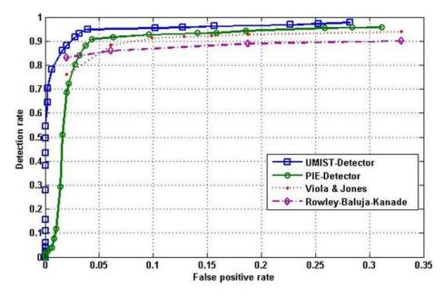
Fig. 8: The ROC curve of UMIST-Detector, PIE-Detector, and other detectors using the MIT-CMU test base.
