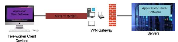
Figure 2: Tunneling Architecture
