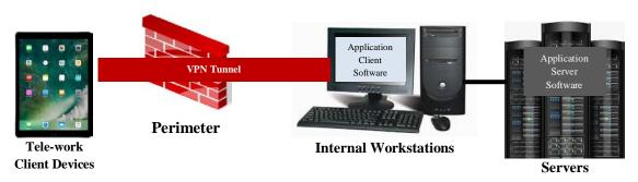
Figure 4: Remote Desktop Access Architecture
