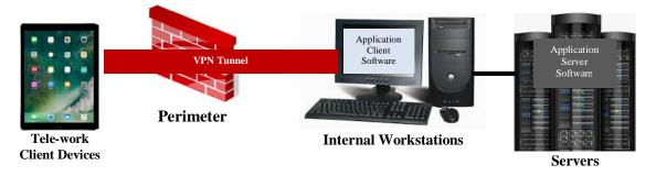
Figure 5: Direct Application Access Architecture
