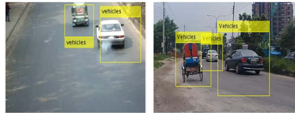
Fig. 3: Left: Detected vehicles from video taken from over bridge, Right: Detected vehicles from a video taken from the side of the road
