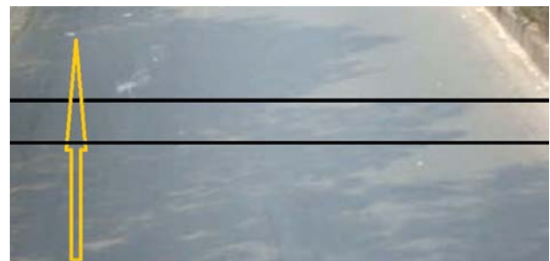
Fig. 4: Two virtual detection lines of a frame. Arrow indicates the flow of traffic
