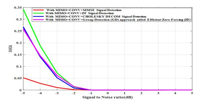
*Fig. 2:* BER performance of encrypted text message transmission through <sup>1</sup>/<sub>2</sub>-rated convolutional channel encoded multi-level CSK modulation scheme aided wireless communication system under implementation of MMSE, ZF, Cholesky decomposition and Group Detection (GD) approach aided Efficient Zero-Forcing (ZF) signal detection techniques.
