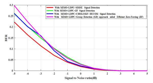
*Fig.3:* BER performance of encrypted text message transmission through LDPC channel encoded multi-level CSK modulation scheme aided wireless communication system under implementation of MMSE, ZF, Cholesky decomposition and Group Detection (GD) approach aided Efficient Zero-Forcing (ZF) signal detection techniques.
