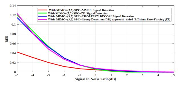
*Fig. 5:* BER performance of encrypted text message transmission through (3,2) SPC channel encoded multi-level CSK modulation scheme aided wireless communication system under implementation of MMSE, ZF, Cholesky decomposition and Group Detection (GD) approach aided Efficient Zero-Forcing (ZF) signal detection techniques.
