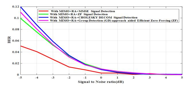
*Fig. 4:* BER performance of encrypted text message transmission through Repeat and Accumulate channel encoded multi-level CSK modulation scheme aided wireless communication system under implementation of MMSE, ZF, Cholesky decomposition and Group Detection (GD) approach aided Efficient Zero-Forcing (ZF) signal detection techniques.
