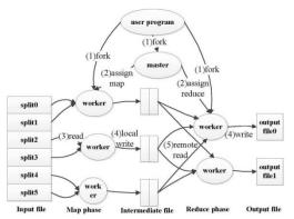
Fig. 1: The framework of the Map Reduce Model
