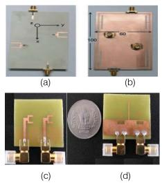
*Fig. 2:* Illustration of integrated MIMO antenna design (a) top view (b) bottom view [10] (c) top view (d) bottom view [11].
