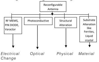
Fig. 6: Reconfigurable antenna various techniques.
