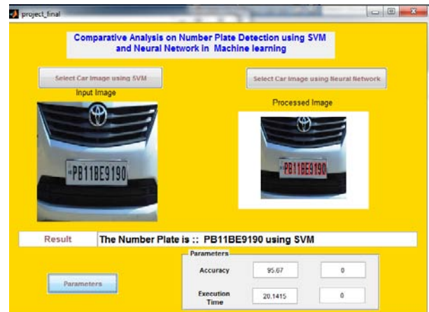
Fig. 10: GUI with results after detection of number plate using SVM.
