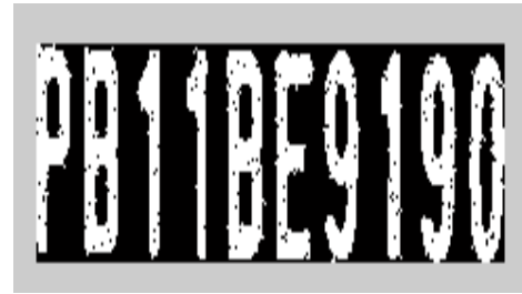
Fig. 9: Cropped Image after plate localization.
