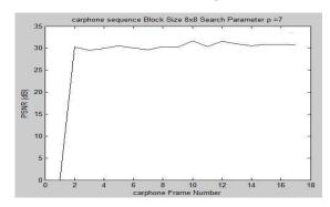
Fig. 11: PSNR of the motion compensated image w.r.t. original image vs Frame Number in NCDS Algorithm
