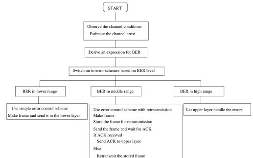
Figure 1: Channel adaptive error control scheme
