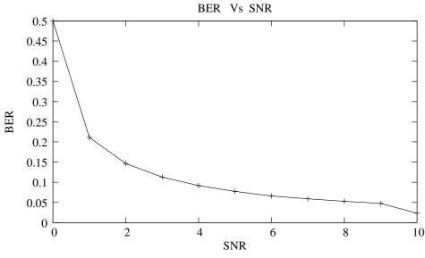
Figure 5: BER Vs. SNR for BPSK
