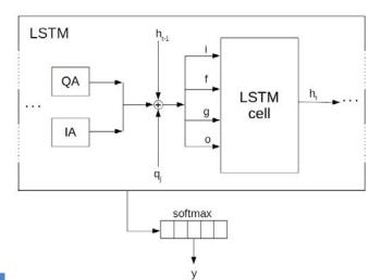
*Fig. 2:* Data flow for LSTM cells inside the LSTM network. Question attention (QA), image attention (IA), previous LSTM state  $(h_{t-1})$  and current question token  $(q_j)$  are used in each LSTM cell gate to generate the context  $(h_t)$  that will be used by the next LSTM cell. A *softmax* classifier is used at the end as the output of the LSTM network to generate one by one each answer word y
