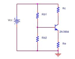
*Figure 2:* The dc equivalent circuit of a common emitter amplifier with ideal capacitors
