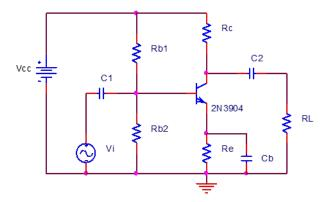
Figure 1: Common emitter amplifier circuit
