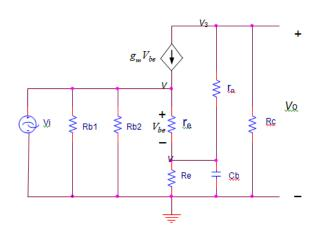
*Figure 5:* The T-model is used here in order to address the finite bypass capacitance Cb
