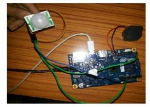
Figure 9 : PIR sensor and Buzzer interfaced with Intel Galileo Gen2
