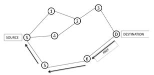
Figure 4 : Propagation of Route Reply (RREP) packet
