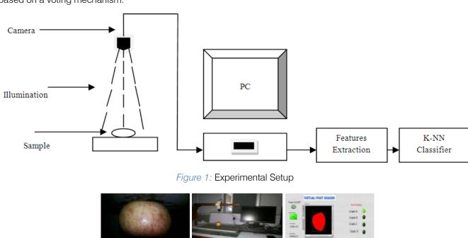
Figure 2: System Overview Block Diagram (a) Fruit Under Inspection (b) Experimental setup (c) Virtual Fruit Grader
