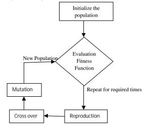
Figure 1 : Flow Chart for normal Genetic Algorithm
