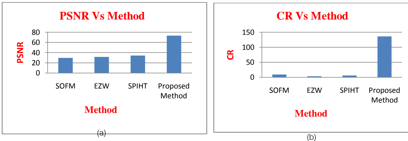
Figure 8 : comparison of various methods with proposed method: (a) PSNR vs Method, (b) CR vs Method
