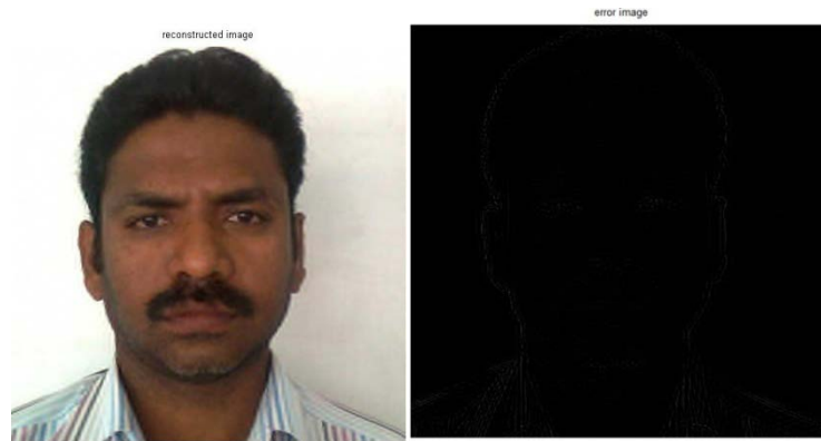
d) With .2 & .4 threshold, 14 x14 block size (e) Error image with .2 & .4 threshold, 14 x14 block size Fig 11: Input, Reconstructed and Error images
