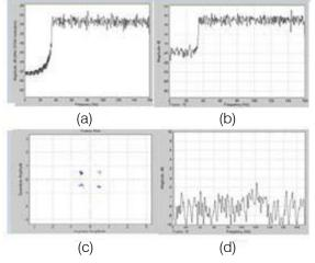
*Figure 5 :* Signal After (a) Modulator Block (b) Before Demodulator (c) Before De-Mapper (d) After De-Mapper
