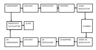
*Figure 2 :* Block Diagram of WiMAX Simulation Model Main subsystems are detailed as:
