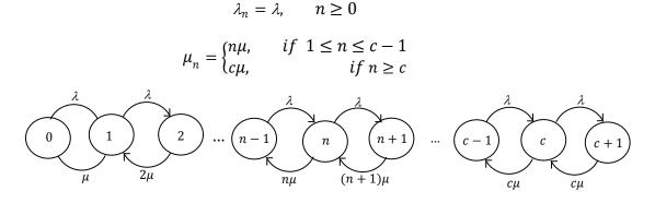
Figure 2.4 : M/M/c Flow Rate [Multiple-ServerCase(c > 1)]
