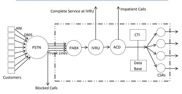
Figure 1.1 : Operational process of an inbound call center
