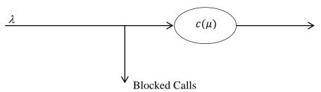
*Figure 2.1* : Description of the M/M/c/c Model and its parameters
