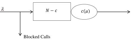
*Figure 2.5* : Description of the M/M/c/N Model and its parameters
