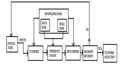
Figure 2 : Block Diagram for Vertical Handoff Decision
