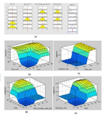
*Figure 4*: (a) IF- THEN rules used in fuzzy block for UMTS to WiMAX; (b) Surface Viewer in case of constant network coverage and QoS; (c) Surface Viewer in the case of constant network coverage and RSSI; (d) Surface Viewer in the case of constant data rate and Qos; (e) Surface Viewer in the case of constant network coverage and data rate.
