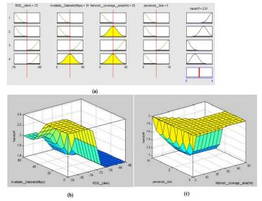
*Figure 5*: (a) IF- THEN rules used in fuzzy block for WiMAX to UMTS; (b) Surface Viewer in the case of constant network coverage and Qos; (c) Surface Viewer for the fuzzy handoff in the case of constant RSSI and data rate
