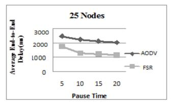
Figure 2(a): Average End-to-End Delay for 25 Nodes
