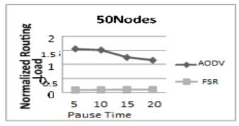
Figure 3(b): Normalized Routing Load for 50 Nodes
