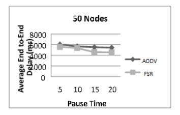
Figure 2(b): Average End-to-End Delay for 50 Nodes
