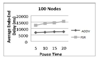
Figure 2(d): Average End-to-End Delay for 100 Nodes
