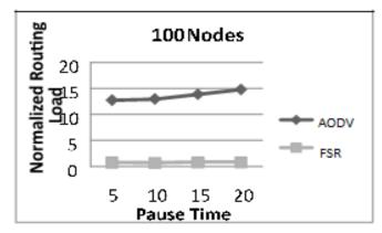
Figure 3(d): Normalized Routing Load for 100 Nodes
