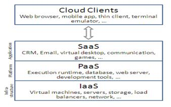
Figure 2: Layers of cloud computing
