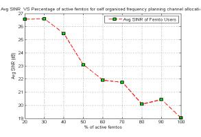
*Figure 7 :* Average SINR Vs Percentage of active femtos for self-organised frequency planning channel allocation
