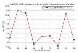
*Figure 3*: Average SINR Vs Percentage of active femtos for orthogonal channel allocation
